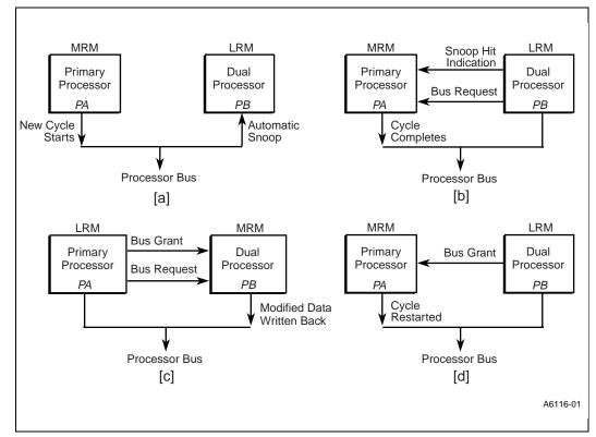
Figure 16-13. Dual Processor L1 Cache Consistency
